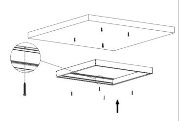
$3.\ Fix semi-finished \emph{f} rame onto ceiling with screw (Concrete ceiling requires plastic anchor)$
